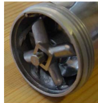
wrong assemble of blade
